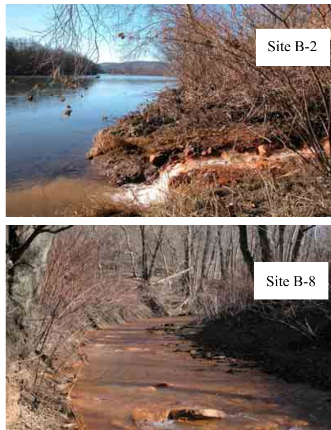
Figure 10. View of significant mine discharge sites B-2 and B-8 identified from TIR data within river reach Sutersville to McKeesport on the Youghiogheny River
